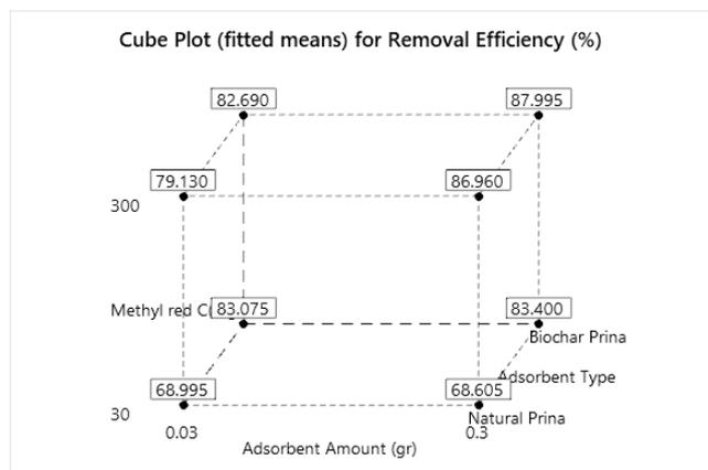
Fig. 2 Cube plot for methyl red removal efficiency
