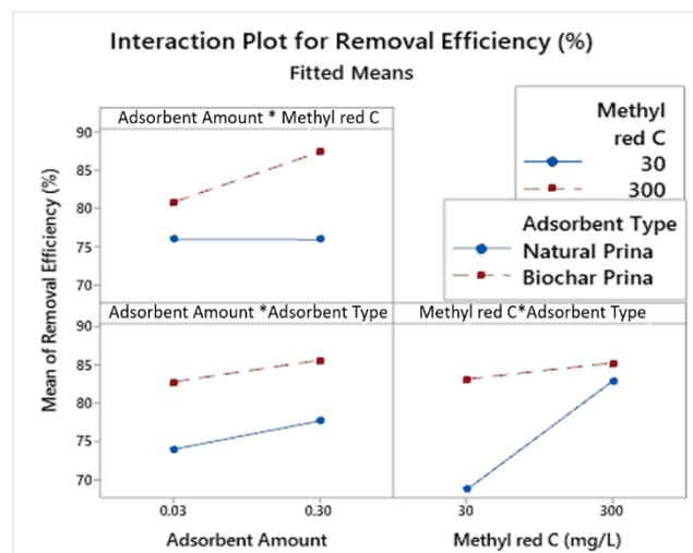
**Fig. 6** Interaction plot for methyl red removal efficiency from aqueous solutions
