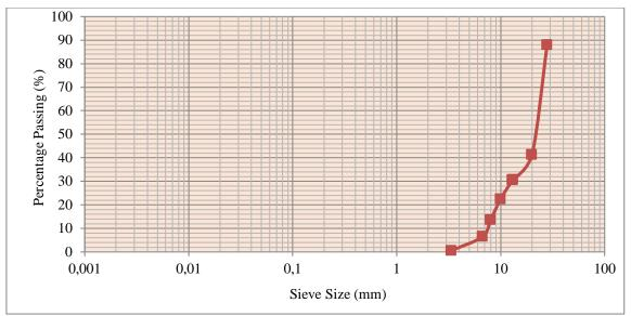
Figure 3. Particle size distribution for coarse aggregate.
