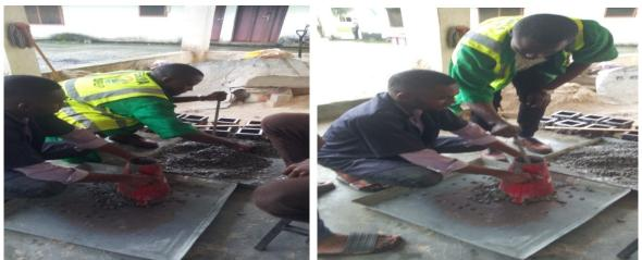
Figure 1. Slump test Experiment.
