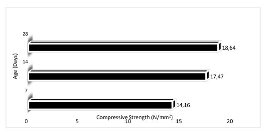
Figure 4. Compressive strength of 3.35-10mm coarse aggregate.
