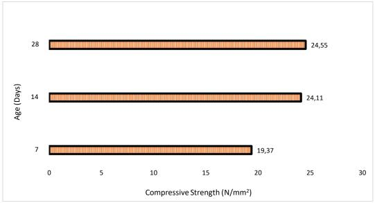
Figure 5. Compressive strength of 13.2-19mm coarse aggregate.
