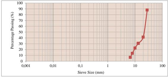
Figure 2. Particle size distribution for fine aggregate.
