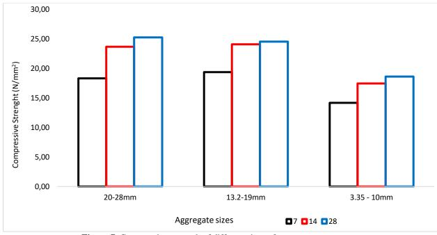
Figure 7. Compressive strength of different sizes of coarse aggregates.
