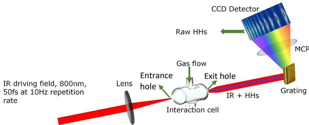
**Figure 1.** Demonstration of the experimental setup of high harmonic generation. CCD: Charged coupled device; HHs: High harmonics; IR: Infrared radiation; MCP: Microchannel plate
