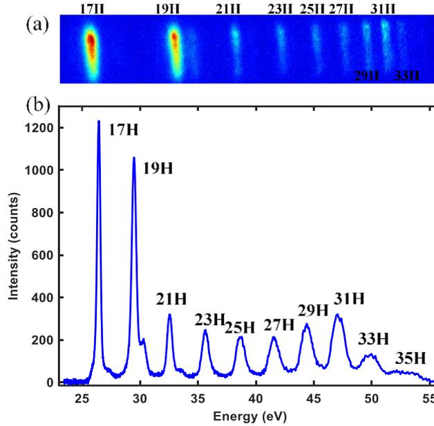
**Figure 3.** The pulse energy of the driving field is 3mJ. (a) Raw data of harmonic spectrum in molecular nitrogen is recorded using CCD camera, (b) Harmonic yield as a function of photon energy (eV)
