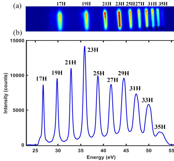
**Figure 2.** The pulse energy of the driving field is 6mJ. (a) Raw data of harmonic spectrum in molecular nitrogen is recorded using CCD camera, (b) Harmonic yield as a function of photon energy (eV)
