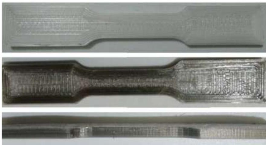
**Figure 4.** Pure Nylon and Nylon + 316L composite printing prepared with grid pattern. (Sample height 100 mm, thickness 4mm. Cross sectional area subjected to tensile force is ~40 mm<sup>2</sup>)
