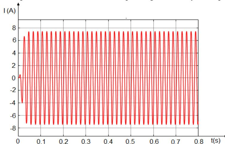
**Figure 15. Load input current (with L filter)**
