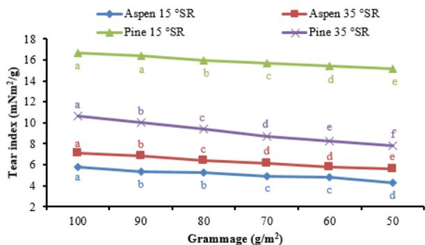
Figure 4. The effect of grammage decreasing on tear index of handsheets in different pulps
