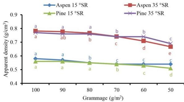
Figure 5. The relationship between grammage and apparent density of handsheets in different pulps
