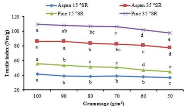
Figure 1. The relationship between grammage and tensile index of handsheets in different pulps (different letters on the same line denote a statistically significant (P > 0.05) difference)
