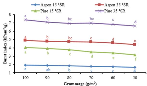
Figure 3. The relationship between grammage and burst index of handsheets in different pulps
