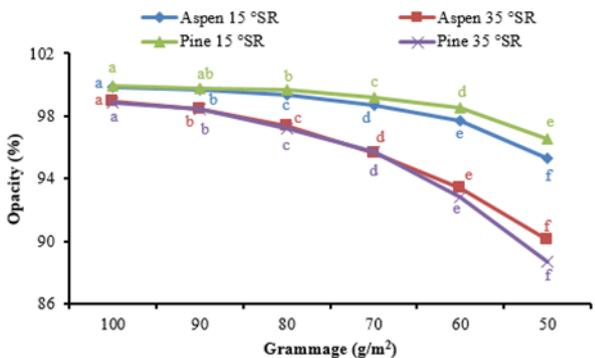
Figure 6. The effect of grammage decreasing on opacity of handsheets in different pulps
