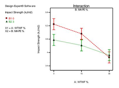
Figure 7: Interaction Graph of WTWF Loading and Addition of MAPE on Impact Strength
