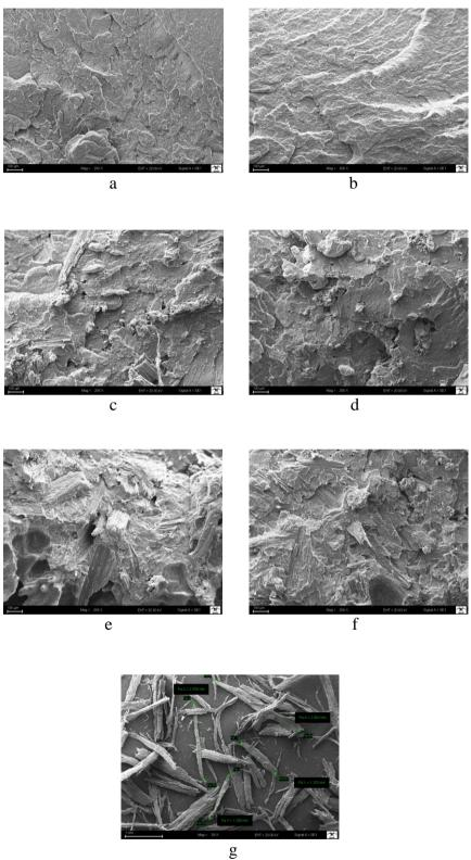
g Figure 10: SEM Micrographs of : (a) HDPE, (b) HDPE + 3% MAPE, (c) HDPE + 15% WTWF, (d) HDPE + 15% WTWF + 3% MAPE, (e) HDPE + 30% WTWF, (f) HDPE + 30% WTWF + 3% MAPE, (g) Waste Tea Wood Fibers.
