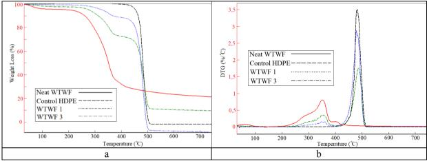
**Figure 8:** (a) TGA Thermographs of Neat WTWF, WTWF Filled HDPE and Control (unfilled) HDPE Thermoplastic Composites; (b) DTG Thermographs of Neat WTWF, WTWF Filled HDPE and Control (unfilled) HDPE Thermoplastic Composites.
