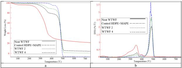
Figure 9: (a) TGA Thermographs of Neat WTWF, WTWF Filled HDPE+MAPE and Control (unfilled) HDPE+MAPE Thermoplastic Composites; (b) DTG Thermographs of Neat WTWF, WTWF Filled HDPE+MAPE and Control (unfilled) HDPE+MAPE Thermoplastic Composites
