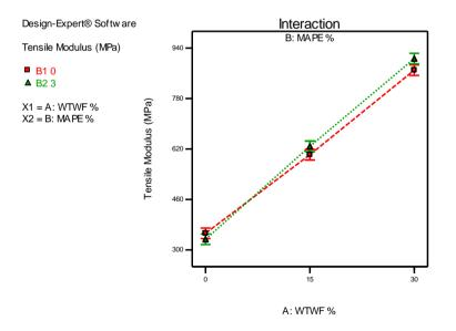
Figure 3: Interaction Graph of WTWF Loading and Addition of MAPE on Tensile Modulus
