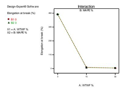
**Figure 4:** Interaction Graph of WTWF Loading and Addition of MAPE on Elongation at Break
