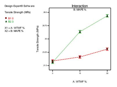
Figure 2: Interaction Graph of WTWF Loading and Addition of MAPE on Tensile Strength
