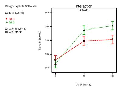
Figure 1: Interaction Graph of WTWF Loading and Addition of MAPE on Density Value
