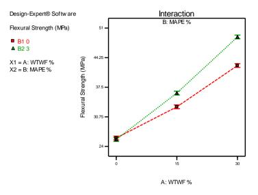
Figure 5: Interaction Graph of WTWF Loading and Addition of MAPE on Flexural Strength
