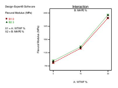
Figure 6: Interaction Graph of WTWF Loading and Addition of MAPE on Flexural Modulus
