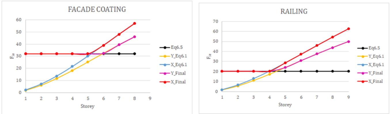
Figure 4.  $F_{ie}$  loads for facade coatings and railings for every floor
