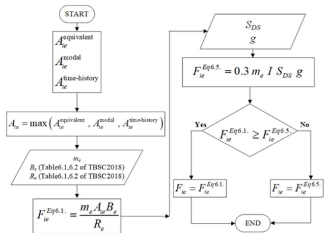
Figure 1. Flow chart of equivalent earthquake load calculation
