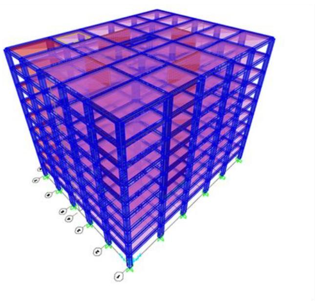
The local soil class was taken as ZD and the earthquake ground motion level as DD-2 from the AFAD (Disaster and Emergency Management Presidency) earthquake map belonging to the coordinates of the ground values (Latitude: 39.344763° Longitude 29.26084°) on which the example model will be constructed. Ground data are shown in Table 2.
