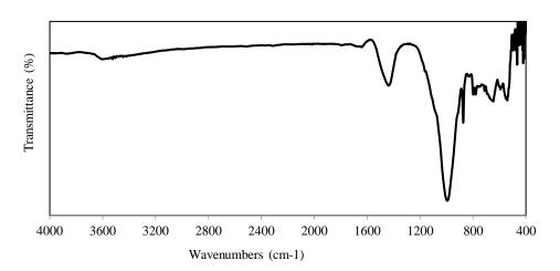
Figure 2. FTIR spectrum of BK adsorbent
