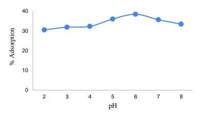
Figure 4. The effect of pH on BK adsorbent of CV dyestuff (adsorbent amount = 0.2 g, concentration =10 mgL<sup>-1</sup>, temperature = 313 K)
