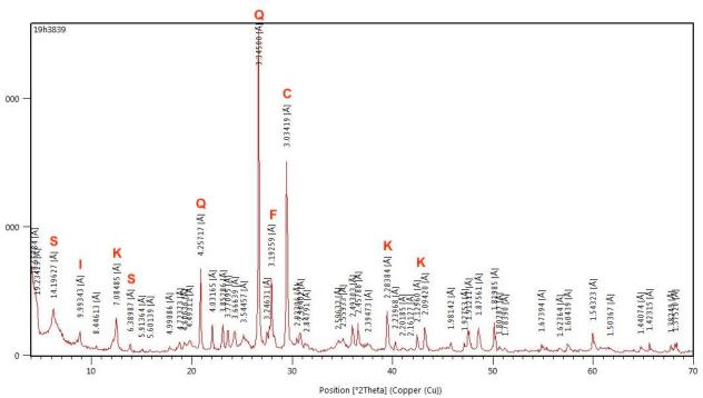
Figure 1. XRD analysis of BK adsorbent (S: Smectite, I: Illite, K: Kaolinite, Q: Quartz, C: Calcite, F: Feldspar)
