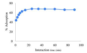
Figure 6. The effect of interaction time on the amount of adsorption (pH:6.0, adsorbent amount = 0.6 g, concentration =  $70 \text{ mgL}^{-1}$ , temperature = 313 K
