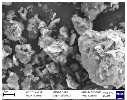
Figure 3. Scanning electron microphotograph of BK adsorbent
