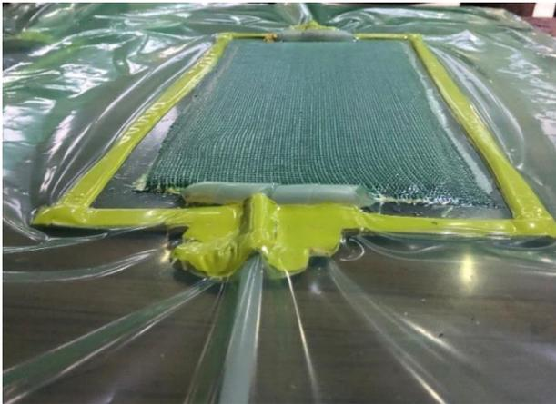
Figure 5 Vacuum assisted resin transfer molding process
