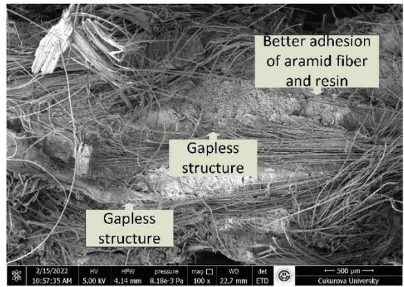
Figure 25 AP composites SEM micrograph
