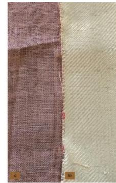
Figure 1 Texture samples: a) Jute texture b) Aramid texture
