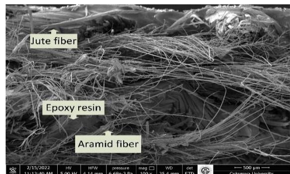
Figure 23 JAV hybrid composites SEM micrograph
