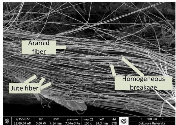
Figure 26 JAP hybrid composites SEM micrograph
