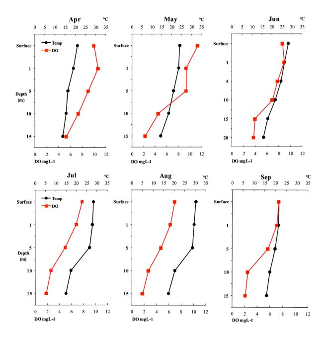
Figure 2. Vertical profiles (every 5 m of depth) of temperature (°C) and dissolved oxygen (mg L<sup>-1</sup>) in KDL.
