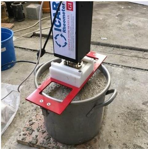
Figure 3. ICAR Testing Instrument
