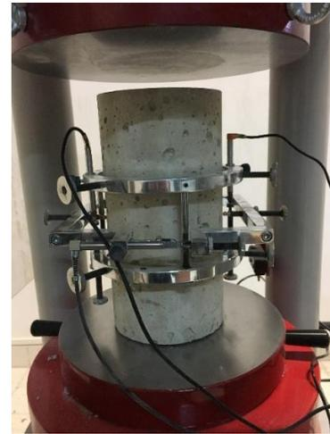
Figure 4. Testing Frame for Compression Testing
