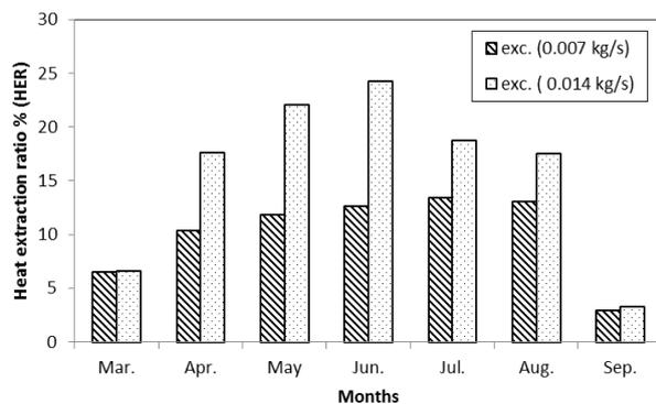
**Figure 9.** Heat extraction ratio for different flow rates
