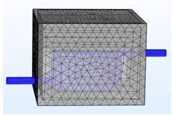
**Figure 2.** Mesh distribution of the solar pond
