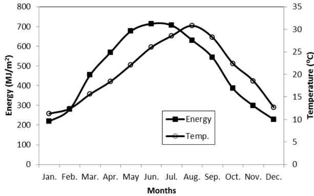
**Figure 3.** The solar energy and ambient temperature distributions for Adana, Turkey, 2010 (Adana Meteorology Regional Office, 2018) Maximum and minimum incident solar energy on the surface of the solar pond is 713.91 MJ/m<sup>2</sup> in June and 218.48 MJ/m<sup>2</sup> in January, and the monthly average maximum and minimum temperatures are observed 30.80 °C in August and 11.30 °C in January, respectively.
