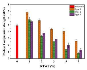
Figure 5 Compressive Strength versus RTWF percentage of CLCM specimens on 28 days curing time
