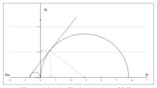
Figure 9 Mohr Circle drawing of LF6
