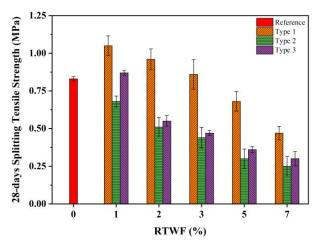
Figure 7 Splitting Tensile Strength versus RTWF percentage of CLCM specimens on 28 days curing time
