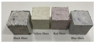
Figure 1 Mortar specimens produced using different colored fibers
