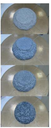
Figure 3 Flow diameter of CLCMs versus RTWF percentage of CLCM specimens
