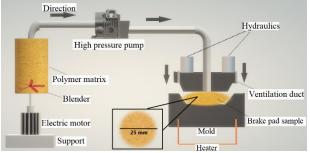
Figure 2. Illustration of sample preparation method
