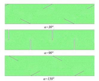
Figure 2. Mesh structures of the numerical model
