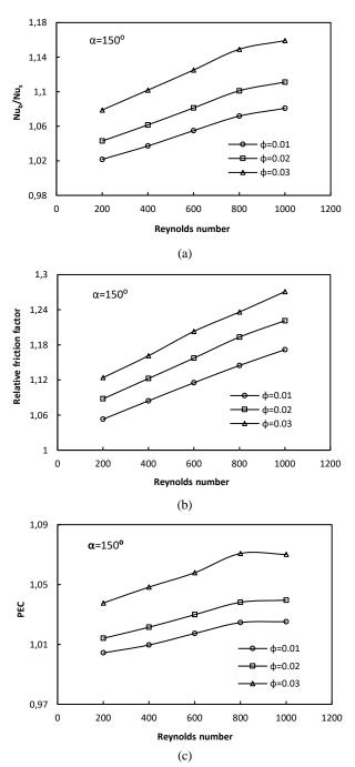
Figure 8. Thermal enhancement factor (a), relative friction factor (b), and PEC (c) with Re and different particle volume fractions at  $\alpha$ =150°
