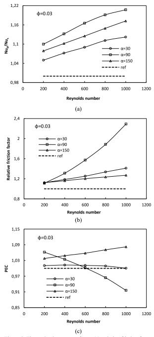
Figure 9. Thermal enhancement factor (a), relative friction factor (b), and PEC (c) with Re and different baffle angles at  $\phi$ =0.03.
