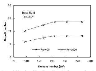
Figure 3. Variation of Nusselt numbers with element numbers for base fluid at Re=600 and Re=1000 ( $\alpha$ =150°)
