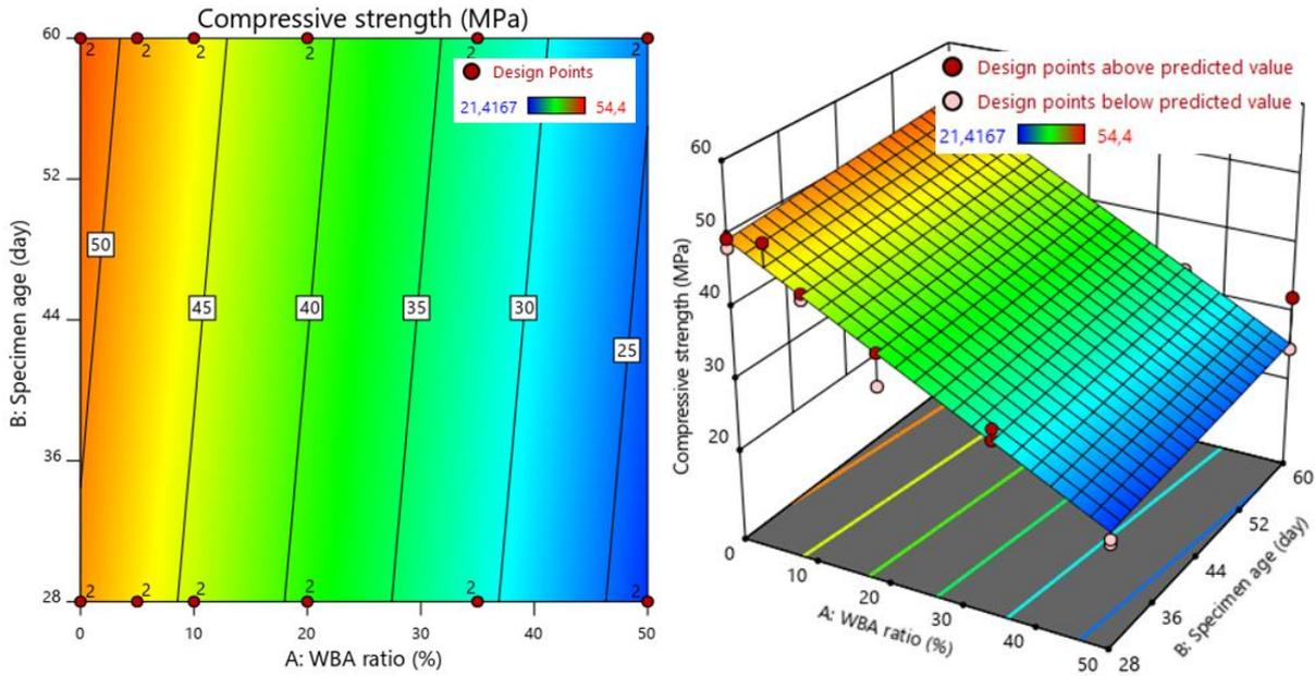
**Figure 9.** Contour and 3D Graphs of Compressive Strength
