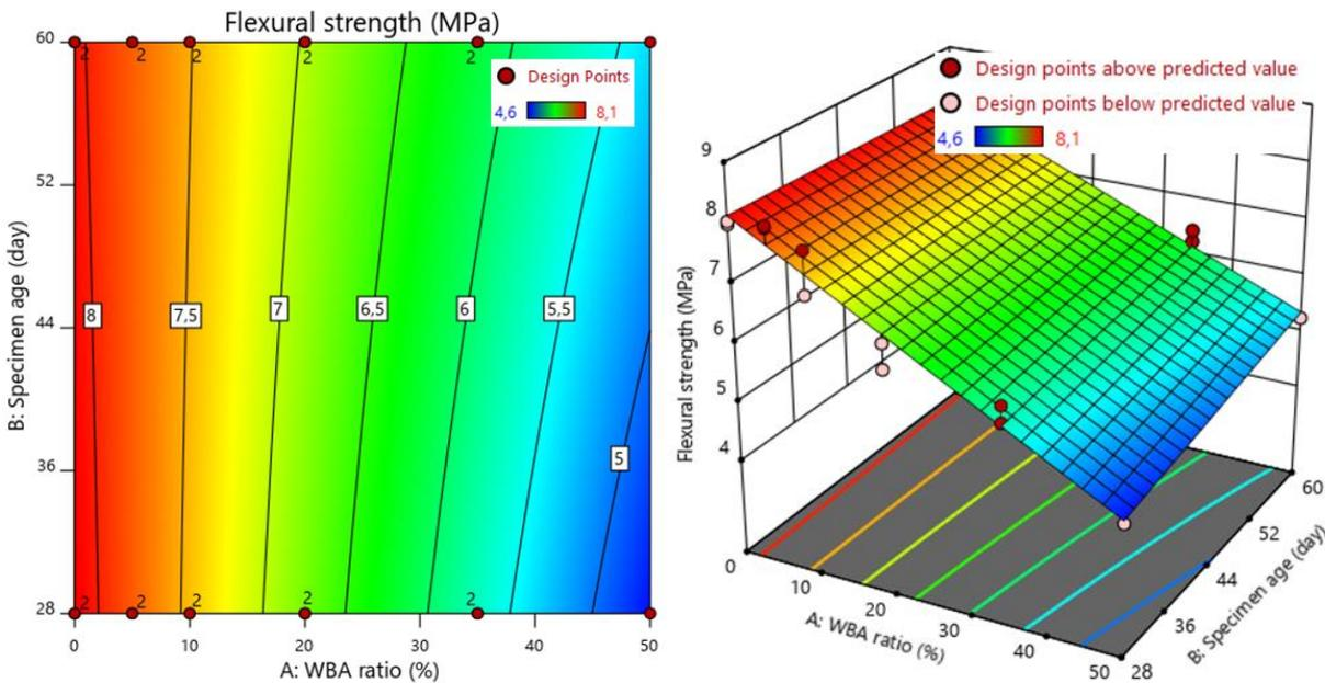
Figure 8. Contour and 3D Graphs of Flexural Strength
