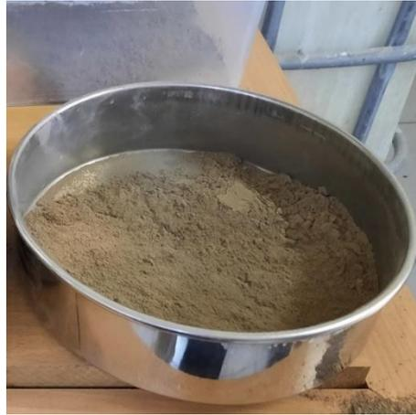
**Figure 2.** Undersize WBA Grains from 75-Micron
