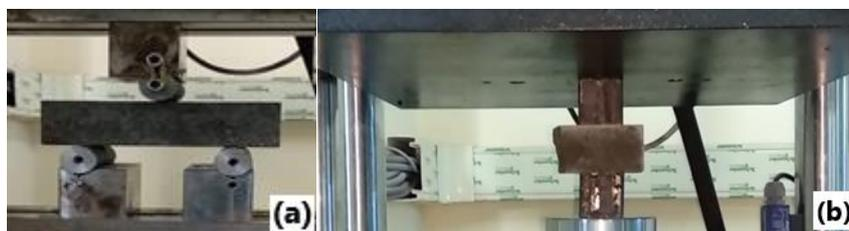
**Figure 5.** Flexural Strength (a) and Compressive Strength (b) Tests
