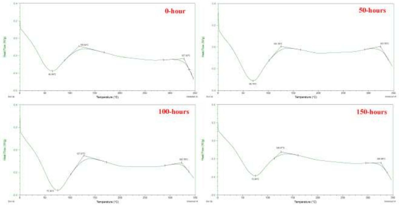
Figure 15. The DSC graphs of coated cotton fabrics
