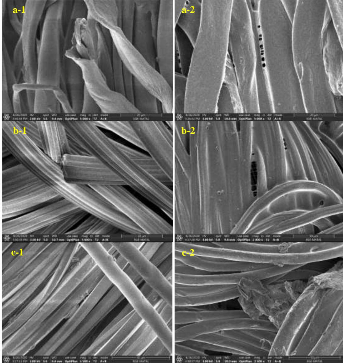
**Figure 2.** SEM images of raw (1) and coated (2) cotton (a), viscose (b), and PET (c) fabrics before UV exposure
