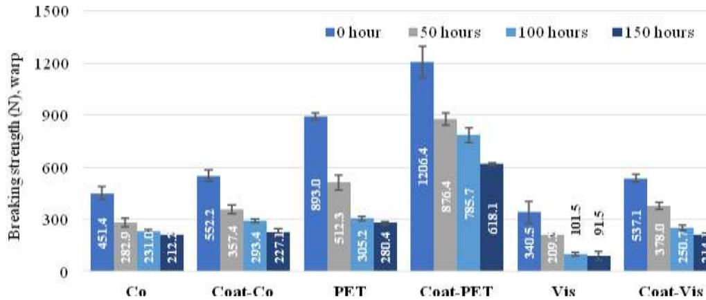
**Figure 3.** Breaking strength of the fabrics (warp direction)
