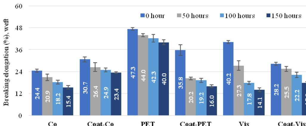
Figure 7. Breaking elongation of the fabrics (weft direction)
