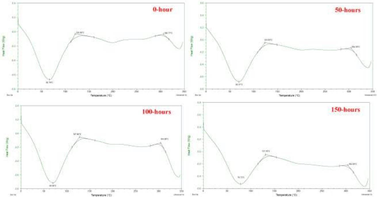
Figure 16. The DSC graphs of coated viscose fabrics
