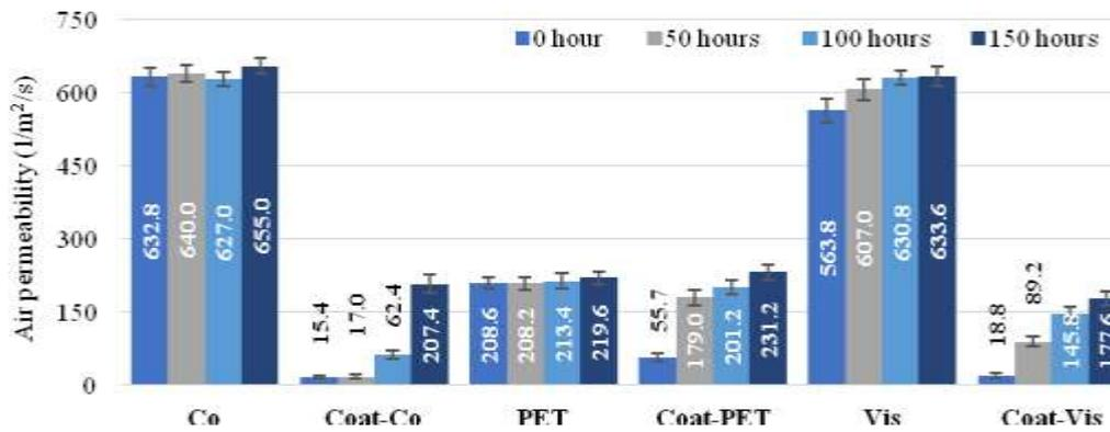
Figure 12. Air permeability of the fabrics
