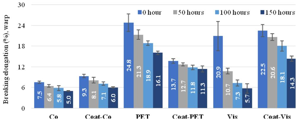
**Figure 6.** Breaking elongation of the fabrics (warp direction)
