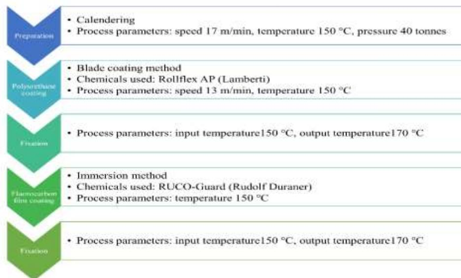
Figure 1. Coating process steps
