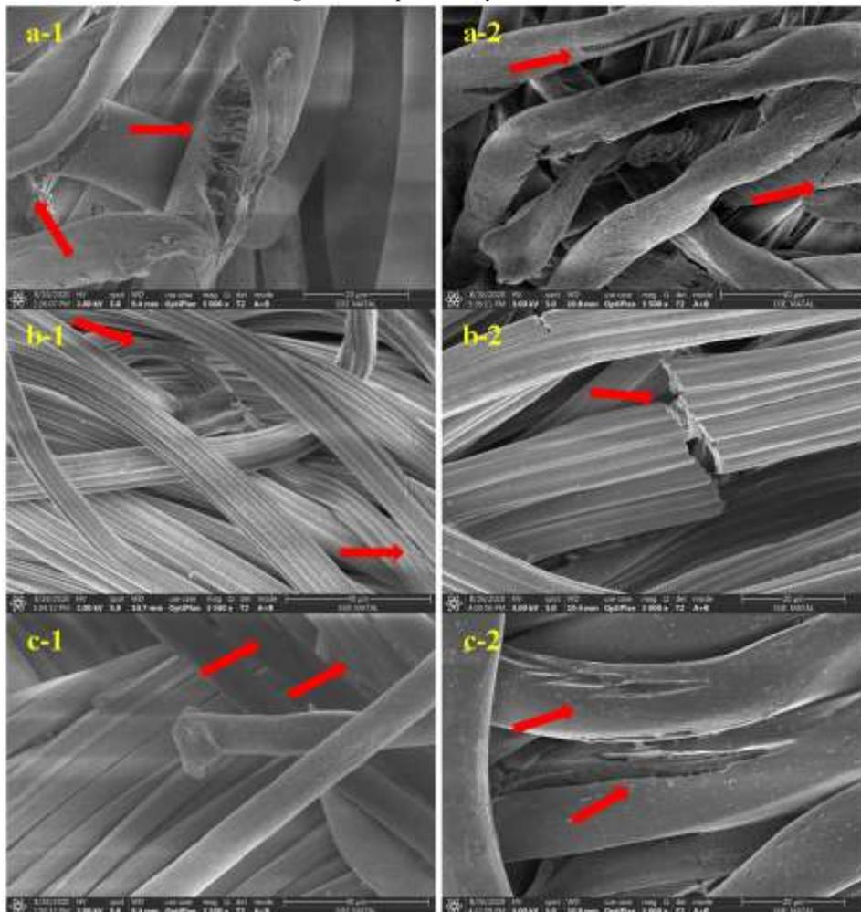
Figure 13. Deep cracks and ruptures observed on the raw cotton (a-1), coated cotton (a-2), raw viscose (b-1), coated viscose (b-2), raw PET (c-1), and coated PET (c-2) fabrics after 150 hours of UV exposure
