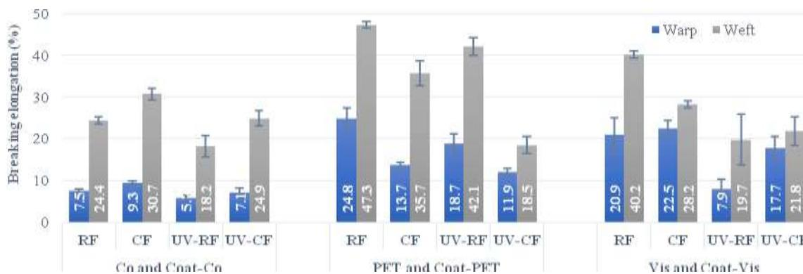
Figure 8. Breaking elongation of raw and coated fabrics independent of UV exposure time
