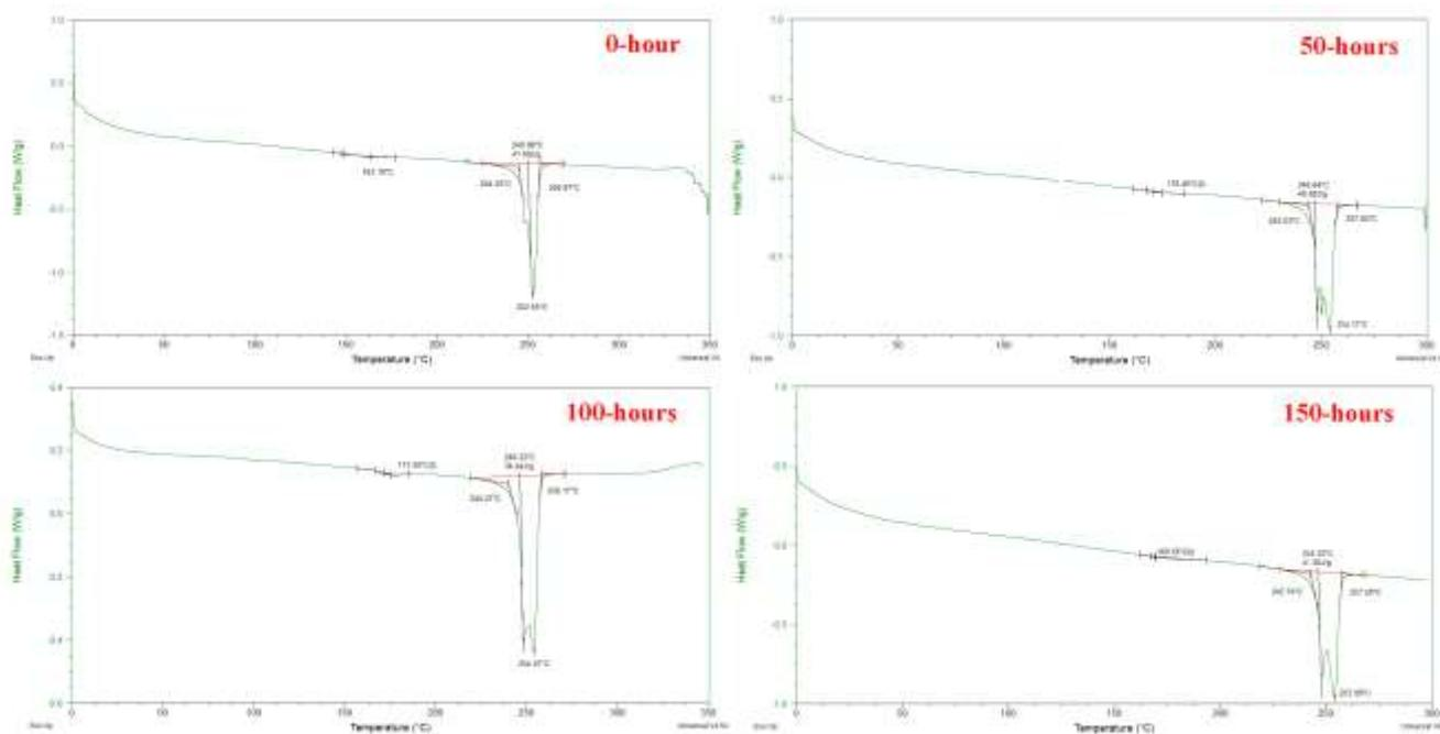
Figure 17. The DSC graphs of coated PET fabrics
