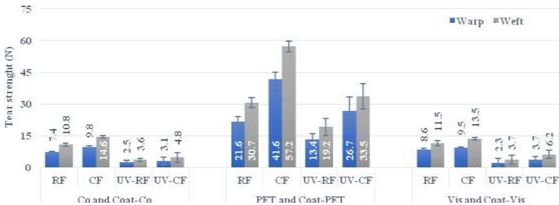
Figure 11. Tear strength of raw and coated fabrics independent of UV exposure time
