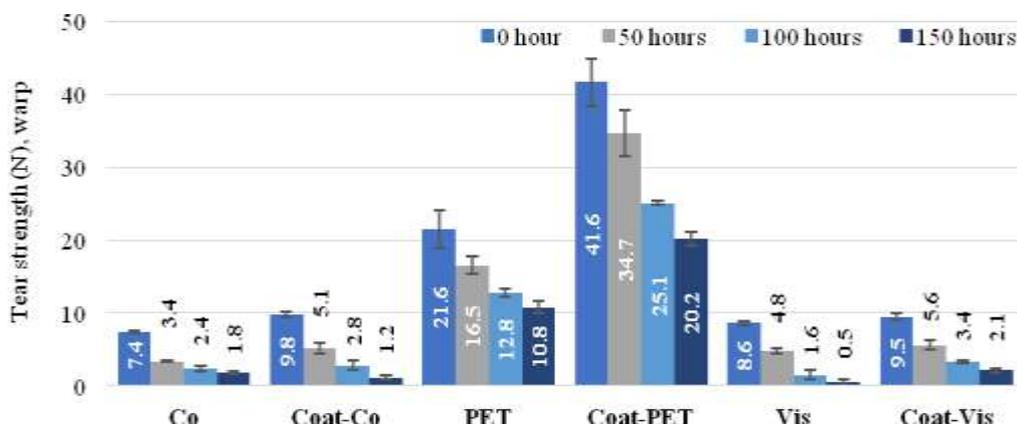
**Figure 9.** Tear strength of the fabrics (warp direction)
