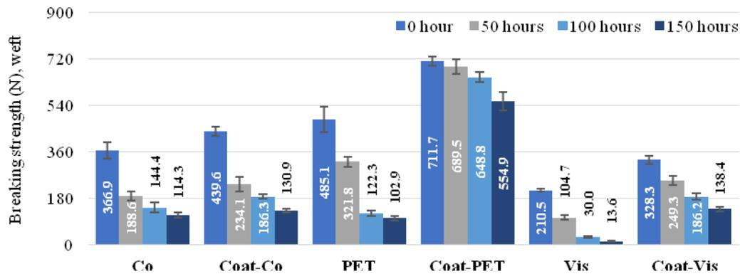
Figure 4. Breaking strength of the fabrics (weft direction)
