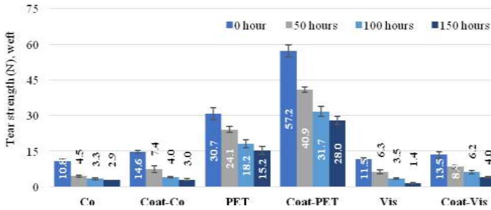
Figure 10. Tear strength of the fabrics (weft direction)
