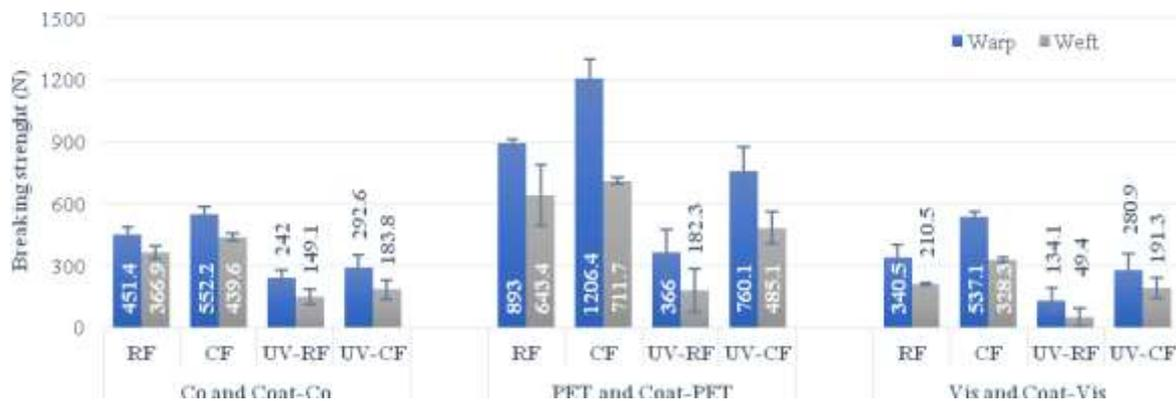
Figure 5. Breaking strength of raw and coated fabrics independent of UV exposure time for all fabric types
