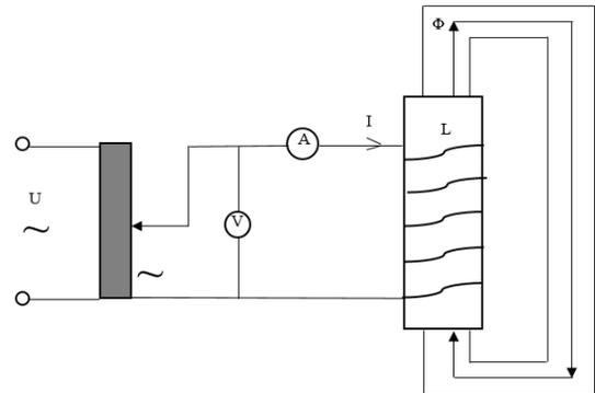
Figure 8. Circuit of the coil with a core in AC
