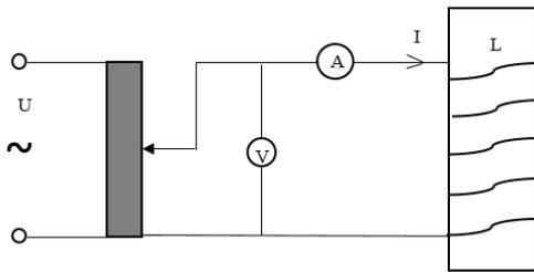
Figure 6. Operation of the coil in coreless AC
