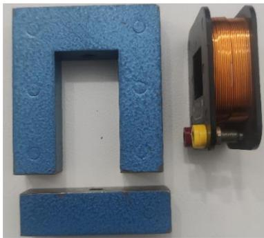
Figure 1. Ferromagnetic core and coil
