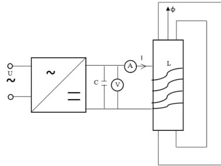
Figure 4. Operation of the coil as a core in DC
