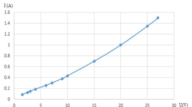
Figure 9. Current-Voltage change of the coil with a core in AC
