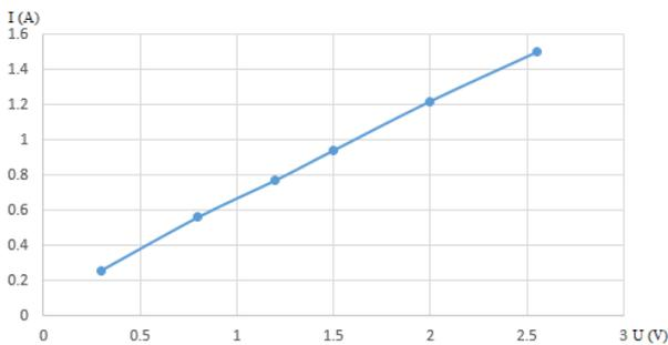
Figure 7. Current-Voltage curve of the coil under AC in coreless condition
