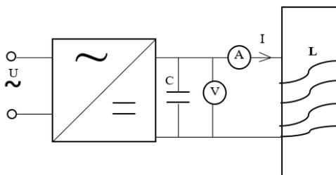
Figure 3. Coil working in DC without core
