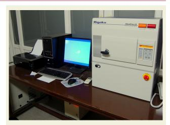
Figure 1. Rigaku Miniflex 2 Benchtop diffractometer
