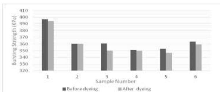
**Figure 4.** The bursting strength results of the fabric samples before and after dyeing
