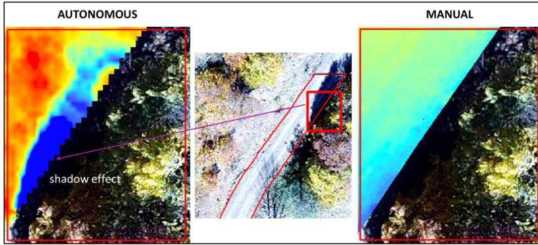
Figure 10. Comparison of autonomous and manual flights in terms of shadow effect
