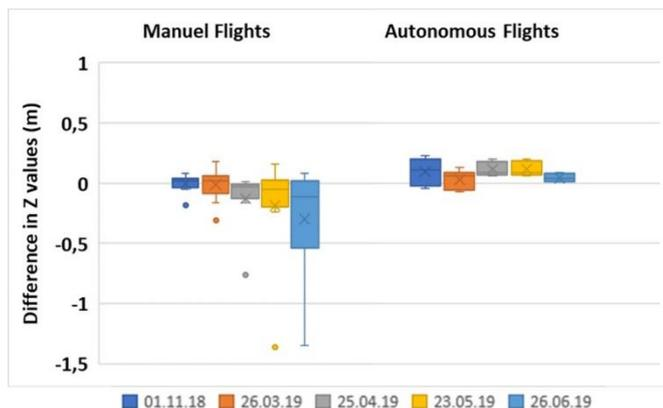
Figure 11. Deformations derived from the average Z-value differences of manual and autonomous flights
