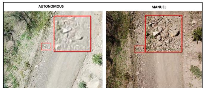
Figure 9. Distinguishability in details based on resolution in images from autonomous and manual flights
