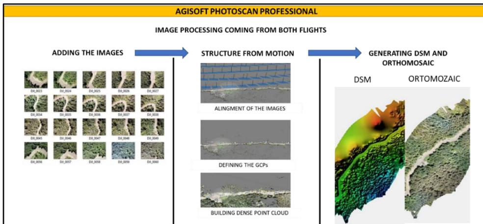
Figure 5. Image processing steps in Agisoft Photoscan Professional version 1.5.2.
