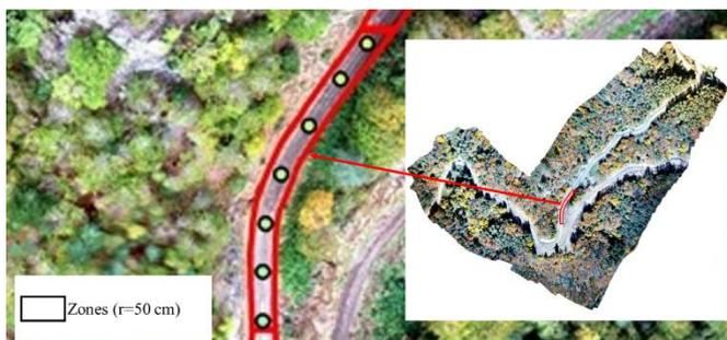
Figure 7. Circular zones with a radius of 50 cm defined on the road surface
