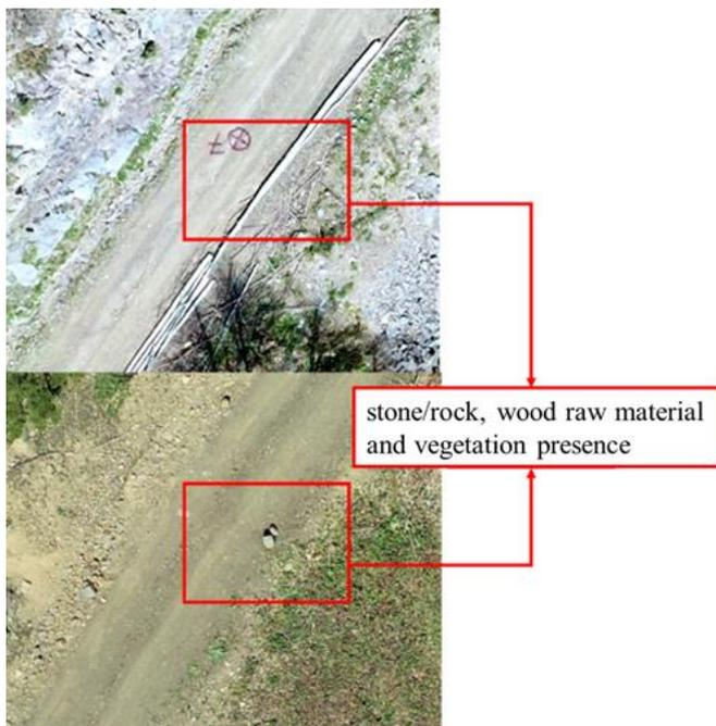
Figure 6. External factors (presence of vegetation, stones/rocks and repair waste)
