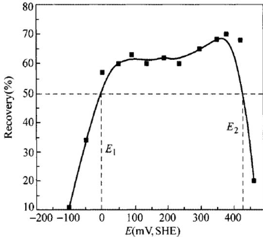
Figure 3. Galenite Recovery versus Pulp Potential (Hu et.al.,2010)
