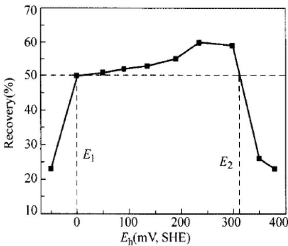
Figure 4. Sphalerite Recovery versus Pulp Potential (Hu et.al., 2010)
