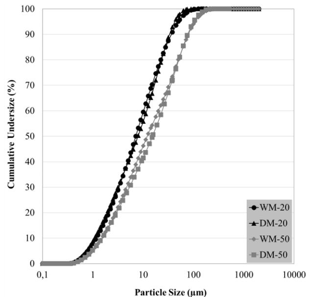
Figure 6. Particle Size Analysis of Samples (Tokcan, 2017)
