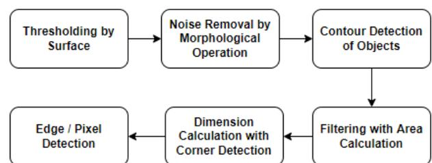
**Figure 5.** Image processing, filtering and size detection flowchart of the object
