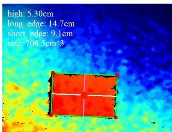
**Figure 7.** Sample product image with 3D dimension calculated
