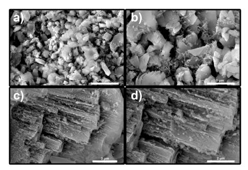
Figure 1. SEM images of g-C<sub>3</sub>N<sub>4</sub> at different magnifications
