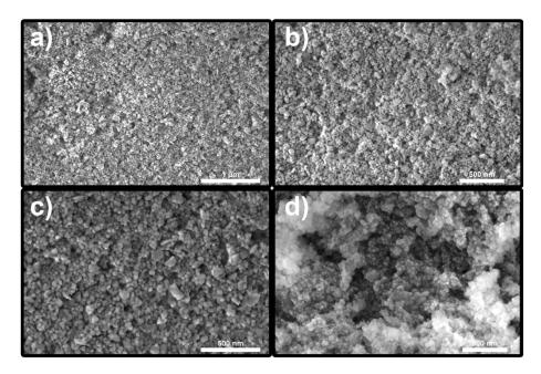
Figure 2. SEM images of ZnS nanoparticles at different magnifications
