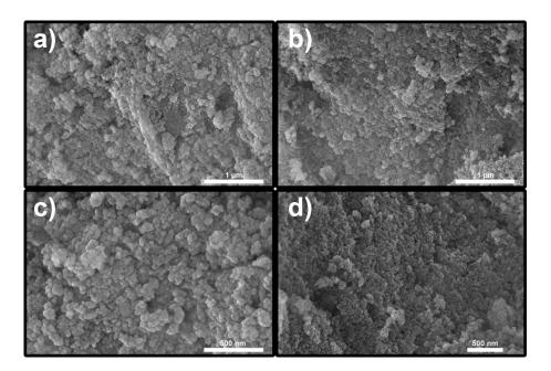
Figure 5. SEM images of ZnS/g-C<sub>3</sub>N<sub>4</sub> 2:1 nanocomposite at different magnifications
