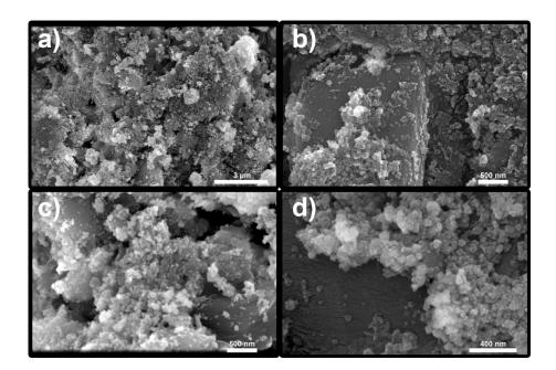
Figure 3. SEM images of ZnS/g-C<sub>3</sub>N<sub>4</sub> 1:2 nanocomposite at different magnifications
