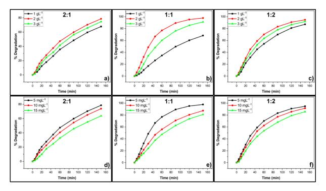
**Figure 7.** The influence of the photocatalyst dosage (a,b,c) and initial dye concentartion (d,e,f) on the photodegradation of RhB
