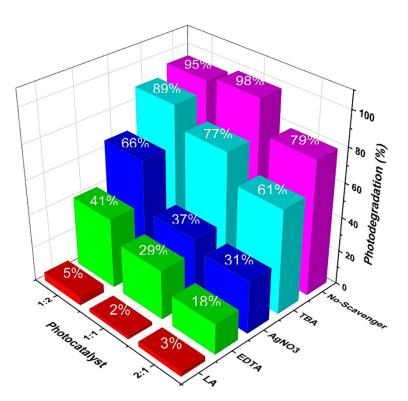
Figure 9. The effects of scavengers on the photodegradation of RhB
