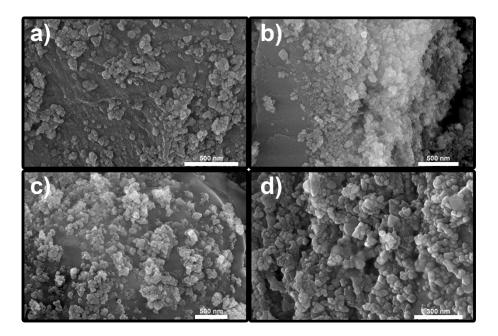
Figure 4. SEM images of ZnS/g-C<sub>3</sub>N<sub>4</sub> 1:1 nanocomposite at different magnifications
