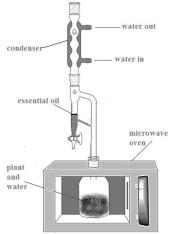
Figure 16. Microwave assisted extraction (Elguea-Culebras et al., 2022)
