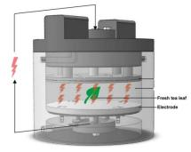
Figure 17. Pulsed electric field extraction schematic diagram (Liu et al., 2019)
