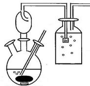
Figure 4. Digestion apparatus (Ashton et al., 1999)
