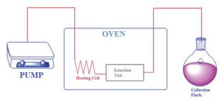
Figure 13. Pressurized liquid extraction system (Alara et al., 2021)
