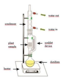
Figure 12. Soxlet assembly (Guntero et al., 2017)
