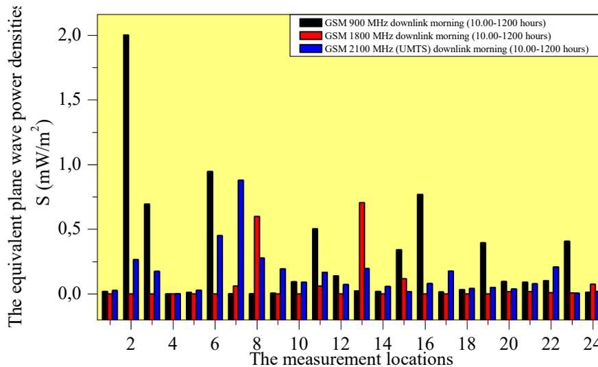
**Figure 5.** The comparison of equivalent plane wave power densities measured at GSM900 MHz and GSM1800 MHz downlink, and GSM2100 MHz (UMTS) frequencies between 10.00-12.00 hours by Aaronia Spectran HF-60105 V4 portable spectrum analyzer.
