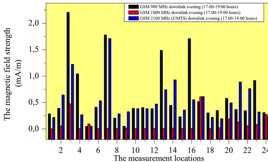
**Figure 7.** The comparison of magnetic field strength measured at GSM900 MHz and GSM1800 MHz downlink, and GSM2100 MHz (UMTS) frequencies between 17.00-19.00 hours by Aaronia Spectran HF-60105 V4 portable spectrum analyzer.
