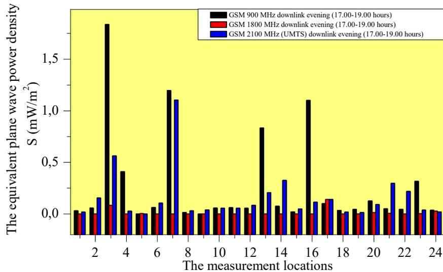
**Figure 8.** The comparison of equivalent plane wave power densities measured at GSM900 MHz and GSM1800 MHz downlink, and GSM2100 MHz (UMTS) frequencies between 17.00-19.00 hours by Aaronia Spectran HF-60105 V4 portable spectrum analyser.
