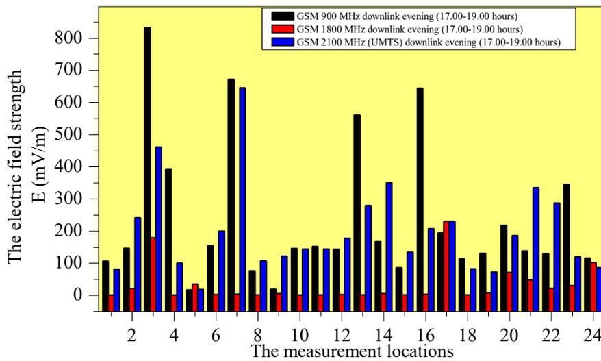
**Figure 6.** The comparison of electric field strength measured at GSM900 MHz and GSM1800 MHz downlink, and GSM2100 MHz (UMTS) frequencies between 17.00-19.00 hours by Aaronia Spectran HF-60105 V4 portable spectrum analyzer.
