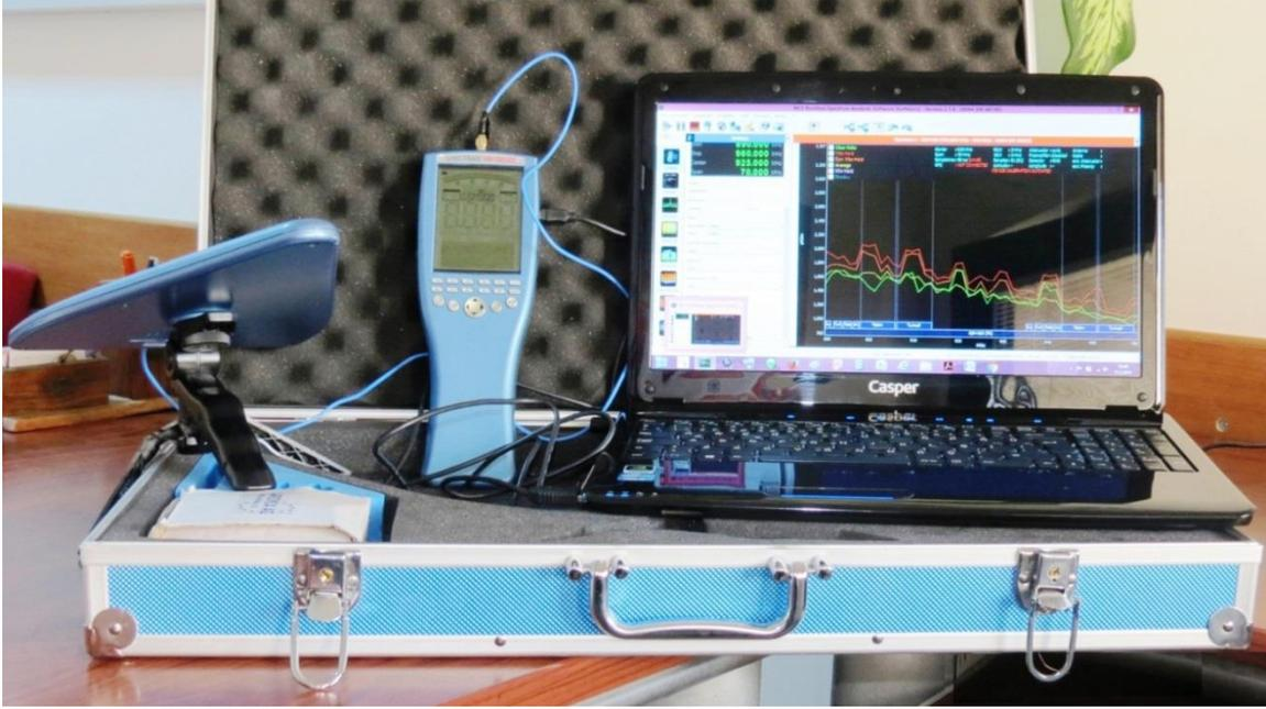
**Figure 1.** Aronia Spectran HF-60105 V4 portable spectrum analyzer and a laptop with MCS software (Sögüt, 2016).
