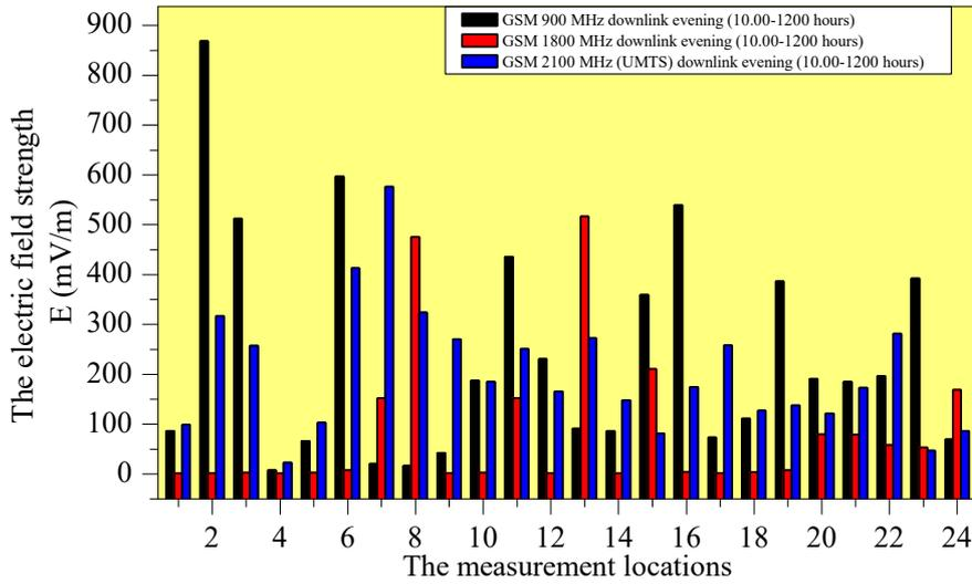
**Figure 3.** The comparison of electric field strength measured at GSM900 MHz and GSM1800 MHz downlink, and GSM2100 MHz (UMTS) frequencies between 10.00-12.00 hours by Aaronia Spectran HF-60105 V4 portable spectrum analyzer.
