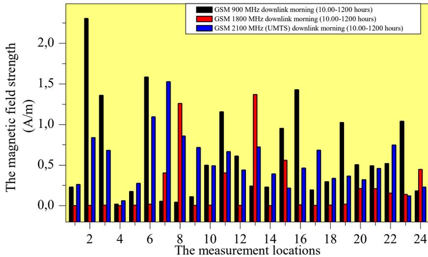
**Figure 4.** The comparison of magnetic field strength measured at GSM900 MHz and GSM1800 MHz downlink, and GSM2100 MHz (UMTS) frequencies between 10.00- 12.00 hours by Aaronia Spectran HF-60105 V4 portable spectrum analyzer.
