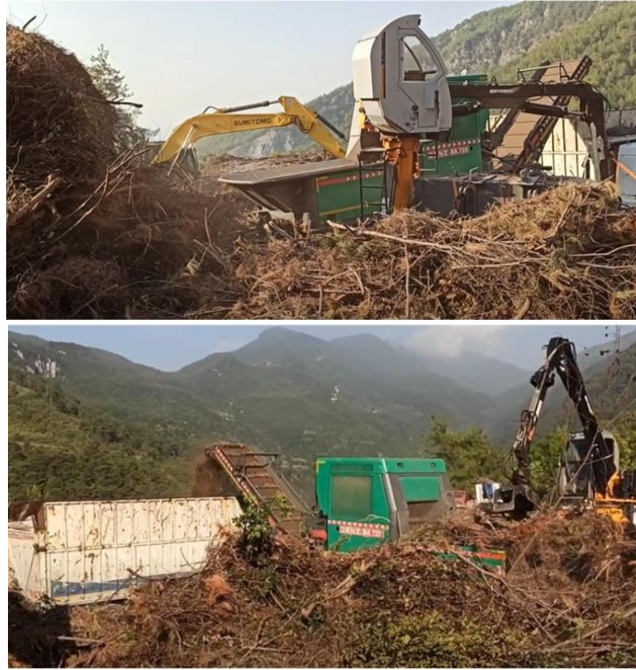
Figure 1. Landing site of a forest residue disposal operation (Erdoğan, 2021)
