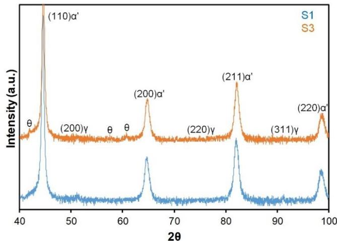
**Figure 2.** XRD patterns of S1 and S3 samples.
