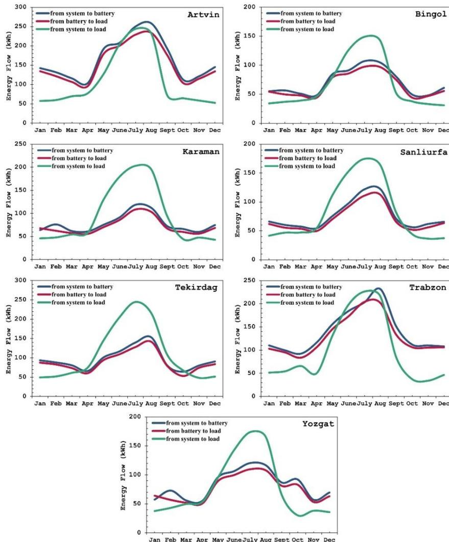
Figure 6. Energy flow in off-grid PV systems
