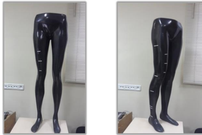
Figure 1. Marked Prosthetic Mould According to ENV 12718 Standard
