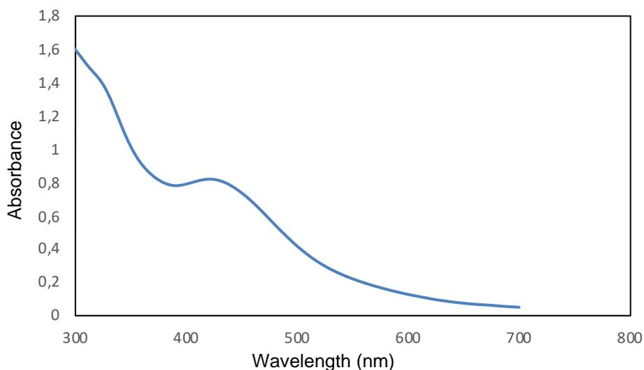
**Figure 1:** UV-Vis spectrum of synthesized Ag NPs
