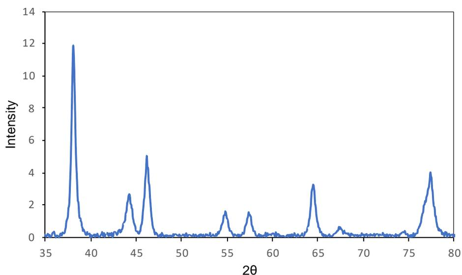
**Figure 2:** XRD spectrum of synthesized Ag NPs
