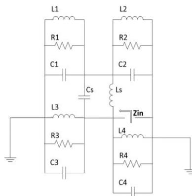
**Figure 3.** Antenna Circuit Equivalent
