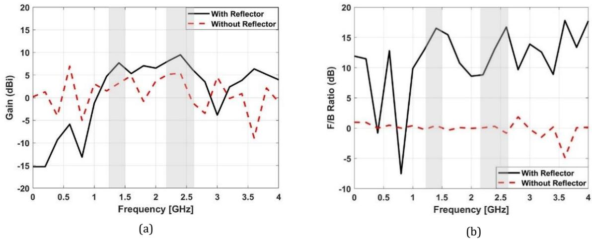
**Figure 6.** (a) Gain simulations of the antenna with reflector and without reflector, (b) The F/B ratio is being analyzed for both the antenna that includes a reflector and the one without a reflector.
