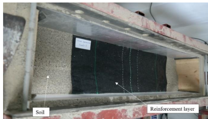
Figure 6. Placement of Sand and Geotextile
