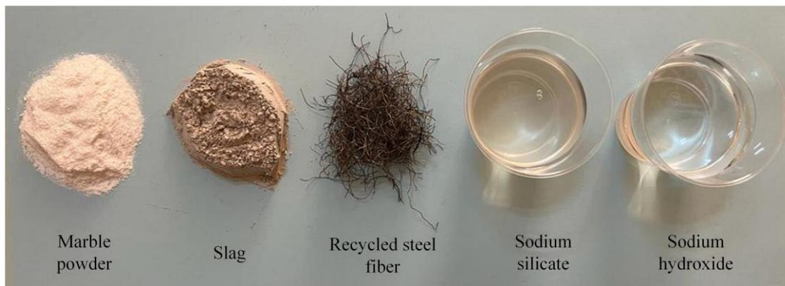
**Figure 1.** Raw Materials Used for Manufacturing Geopolymer Composites
