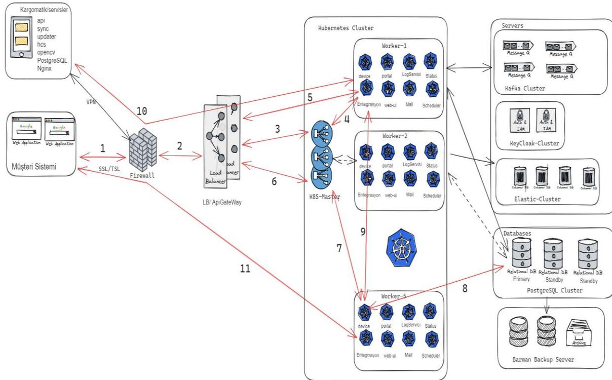
**Figure 19:** The process of transmitting the package information from the e-sales application to the cargo vending machine
