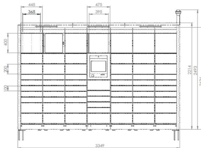
Figure 2: Sizes of the designed cargo vending machine
