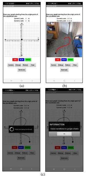
Figure 4. Android application main screen a) drawing on the coordinate axis, b) drawing on the camera image c) information share notes
