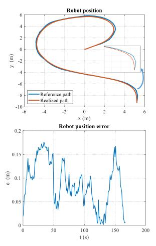
Figure 13. Position control of DDWMR for Lookahead=1 m
