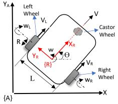
Figure 1. DDWMR motion axis
