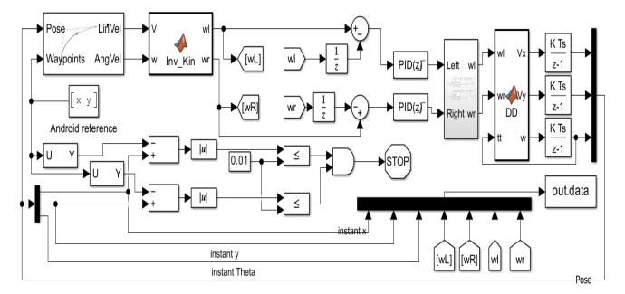
Figure 6. Robot control blocks in Simulink
