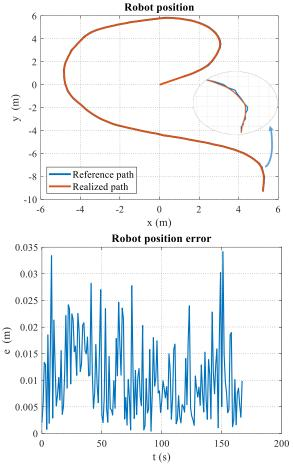
Figure 12. Position control of DDWMR for Lookahead=0.3 m
