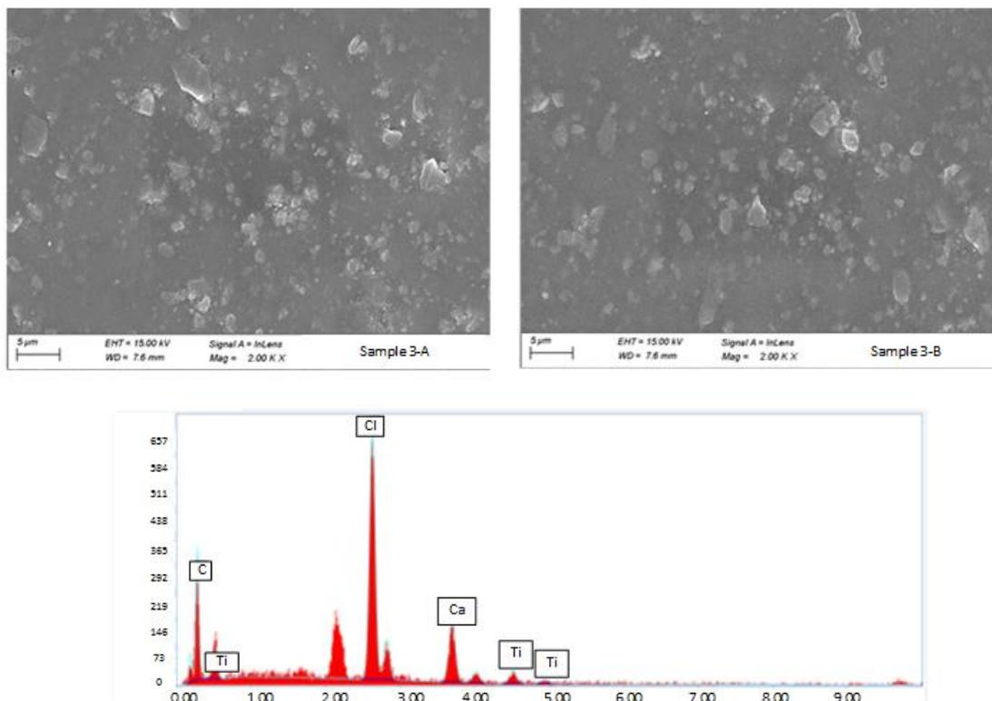
**Figure 8.** SEM images and EDX graph from different locations A and B of sample 3
