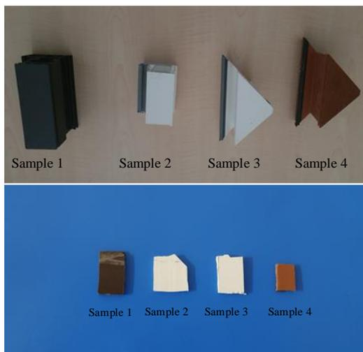
Figure 1. PVC profile samples used in experimental studies
