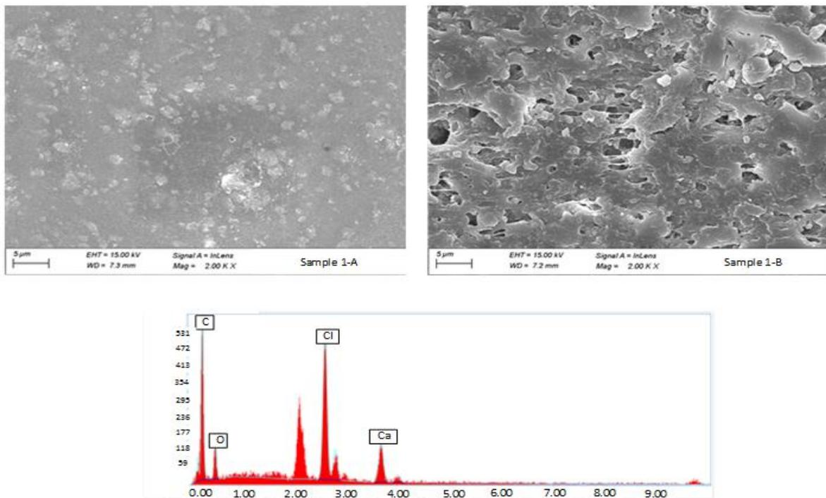
**Figure 6.** SEM images and EDX graph from different locations A and B of sample 1
