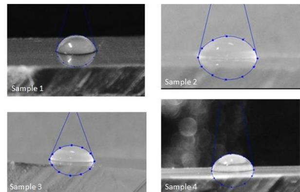
Figure 3. Measuring CAs of 4 samples with the DropSnake measurement method
