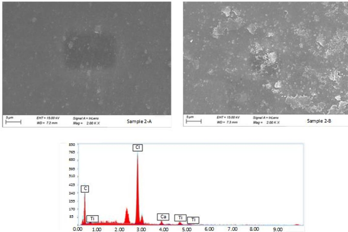
**Figure 7.** SEM images and EDX graph from different locations A and B of sample 2
