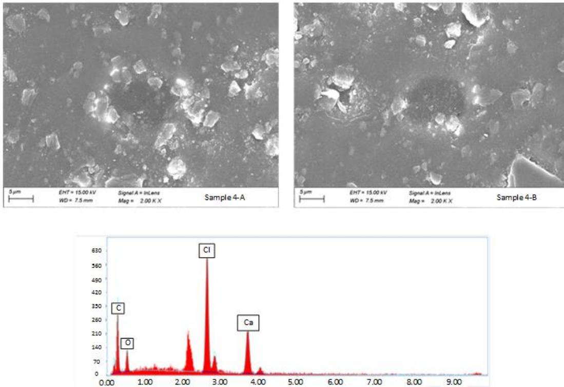
**Figure 9.** SEM images and EDX graph from different locations A and B of sample 4
