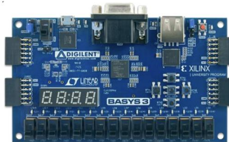
Figure 4. BASYS3 FPGA Training Card Utilized in this Research
