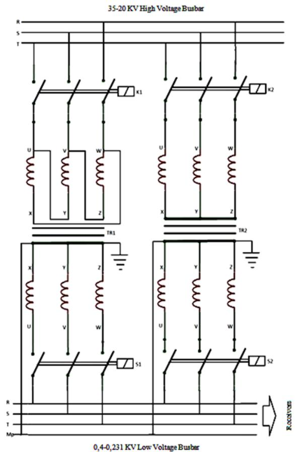
**Figure 2.** Parallel load transfer of transformers
