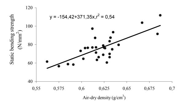
Figure 2. The relationship between static bending strength and air dry density.
