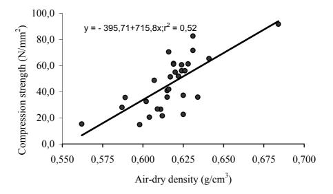
Figure 1. The relationship between compression strength and air-dry density.
