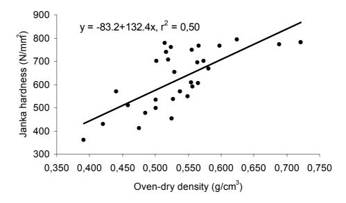
Figure 3. The relationship between janka hardness (cross) and oven - dry density.
