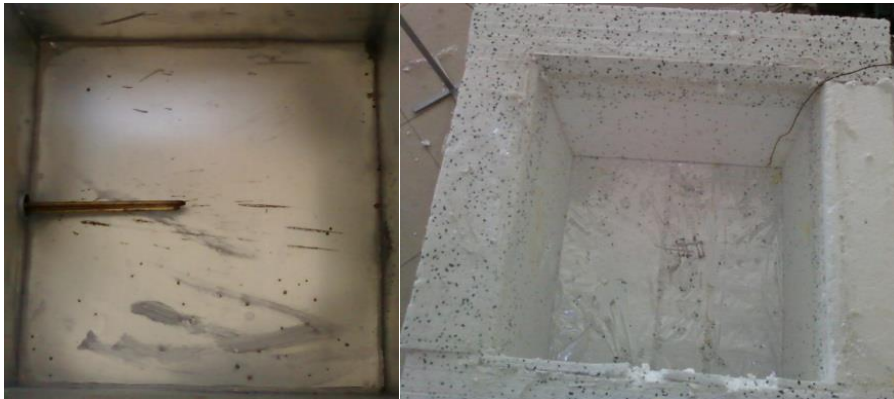
Figure 3 Water Reservoir with Resistance Heater and Placing on The Floor Closed with Aluminum Foil
