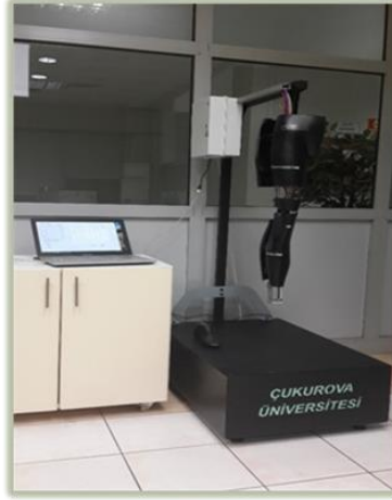
Figure 9. The Final Version of the Prototype Pressure Measurement Device
