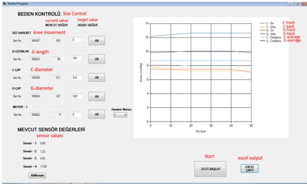
Figure 13. The Final State of the Pressure Values Applied by the Trousers Sample When the Device Becomes Static
