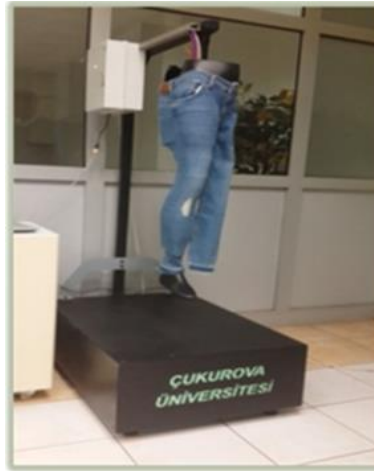
Figure 10. Positioning the Device and Dressing the Lower Body Clothing to be Measured on the Device
