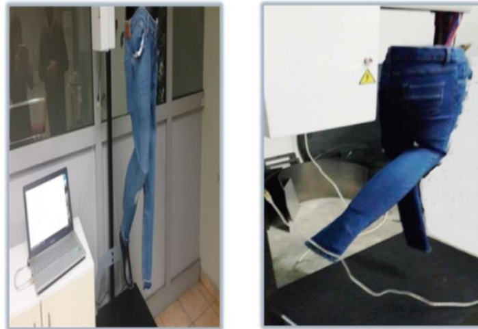
Figure 11. Knee Bending Position of the Pressure Measurement Test Device
