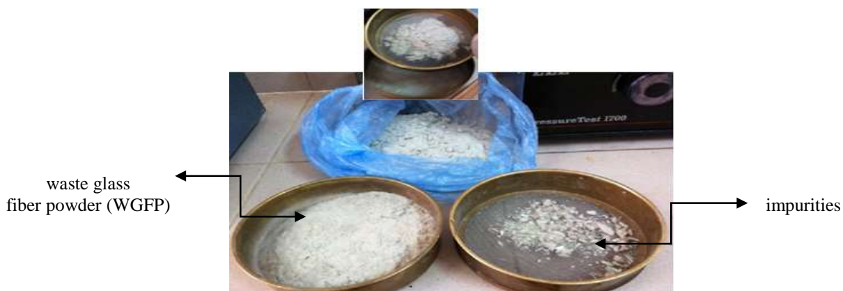
Figure 1. Removing of Coarse Impurities in Waste Glass Fiber
