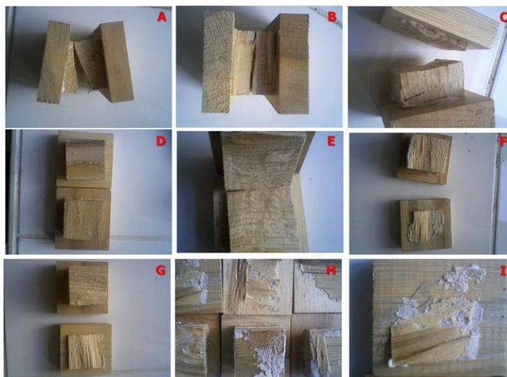
Figure 5. The effects of MW treatment conditions on bonding surface after shear bonding tests (A and B: typical
