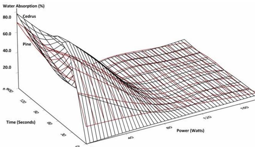
Figure 4. The water absorption (%) properties of MW treated softwoods.
