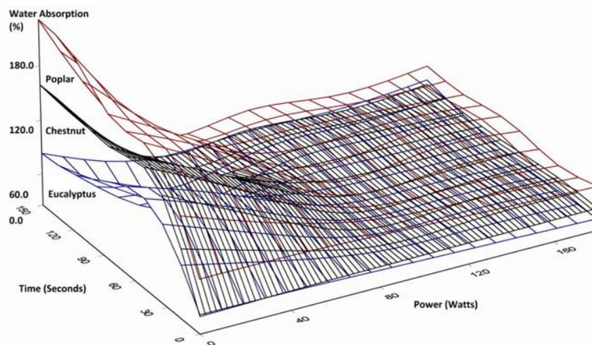
Figure 3. The water absorption (%) properties of MW treated hardwoods.
