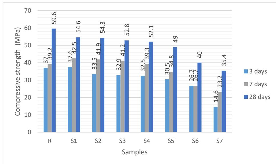
**Figure 5.** 3, 7 and 28-days Compressive strength of the samples
