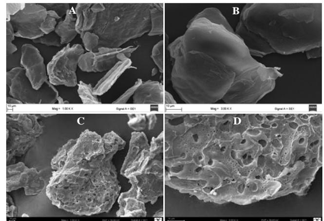
**Figure 4.** SEM images of chitosan with a magnification of (A) 1000 and (B) 3000 times and CMSCh-4; (C) 1000 and (D) 3000 times
