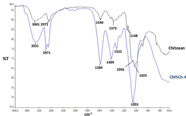
**Figure 5.** FTIR spectra of chitosan and CMSCh-4
