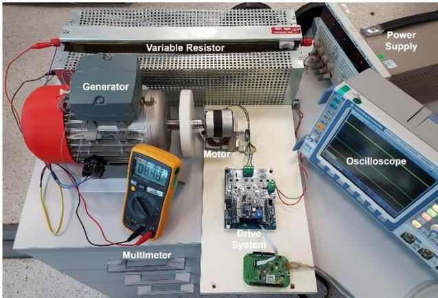
Figure 10 Experimental test setup
