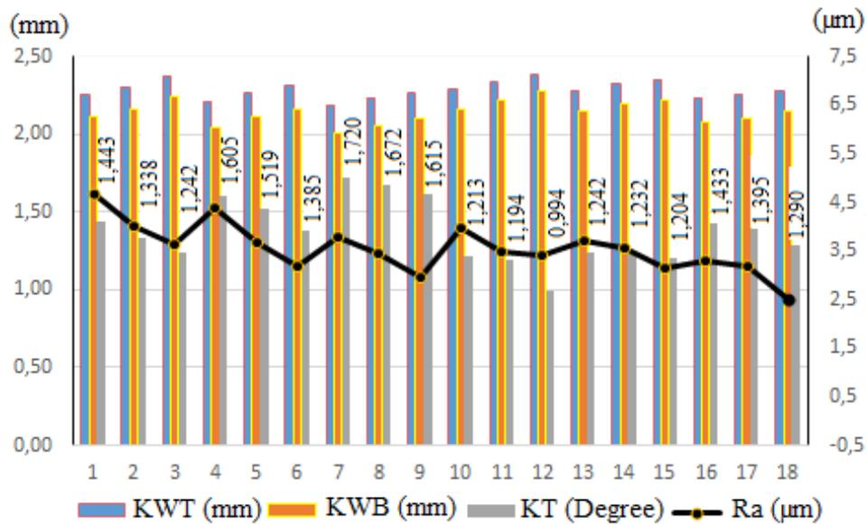
Figure 2. Combined graph of KWT, KWB, KT and Ra
