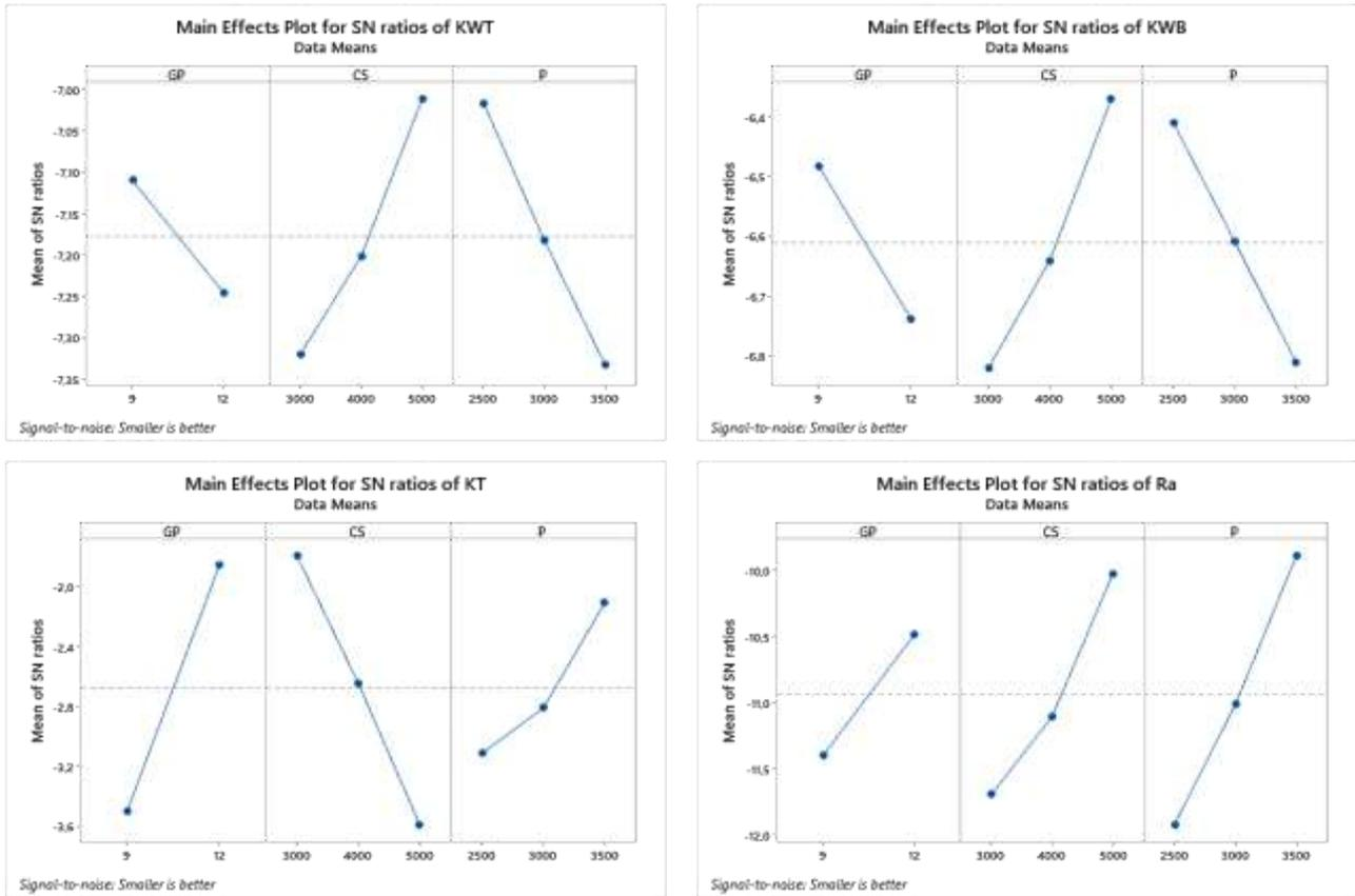
Figure 4. Response graphs for KWT, KWB, KT and Ra
