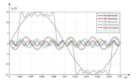
Figure 3. Six-pulse rectifier input current harmonics waveform
