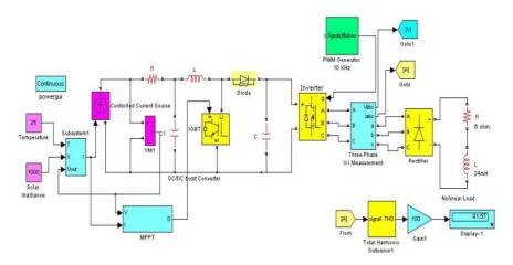
Figure 7. Matlab/Simulink model of stand-alone solar PV system (unfiltered)
