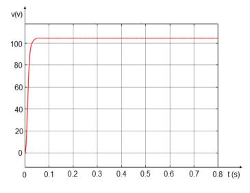
Figure 6. PWM inverter input voltage
