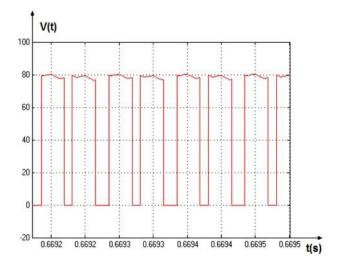
Figure 9. Six pulse uncontrolled rectifier output voltage
