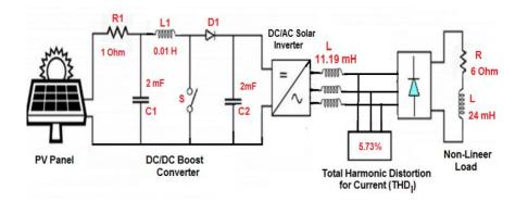
Figure 12. Off-grid PV system model with L filter
