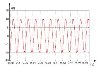
Figure 14. Inverter output current waveform
