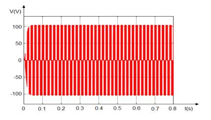
Figure 11. Inverter output voltage waveform
