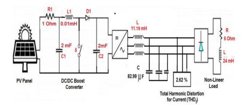
Figure 13. Off-grid PV system model with LC filter
