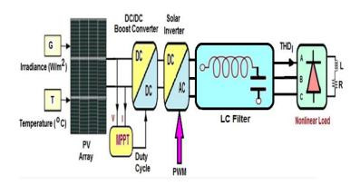
Figure 2. Principle diagram of off-grid PV system (with LC filter)
